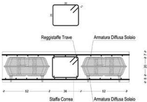
Figure 36 - constructive detail of lightening with stiffening spandrel beam
