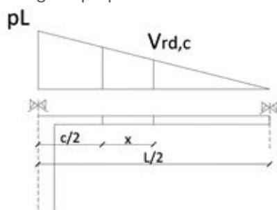
Figura 32 - distance calculation  $x$
