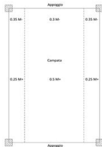
Figura 15 - diagram for the calculation of the design moments - moments of competence of each strip.
