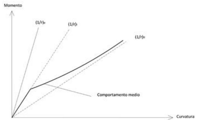
Figure 34 - moment- curvature relation “average” for the calculation of displacements
