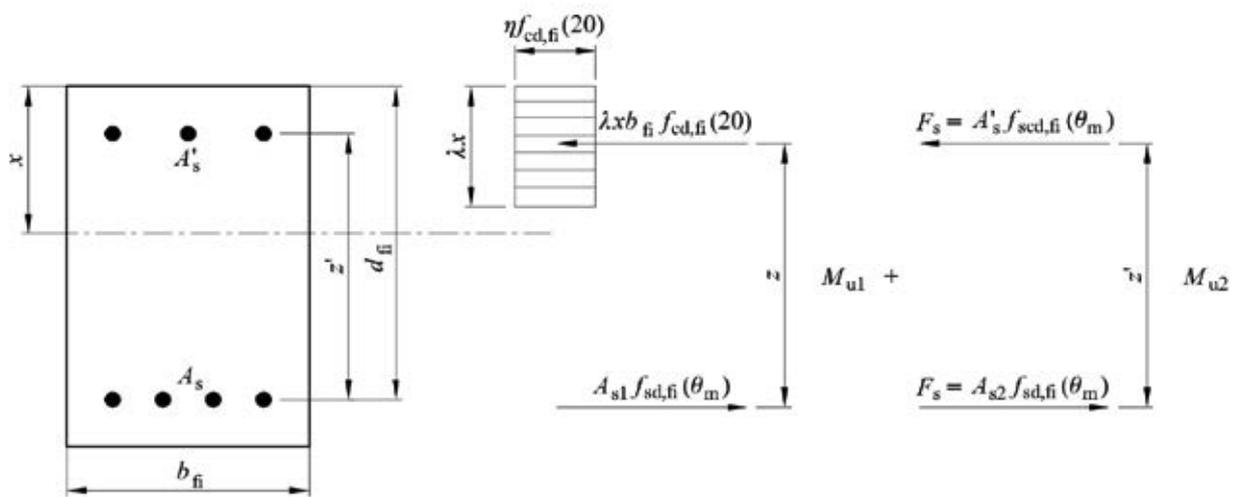
Figure 73 - static scheme for hot verification
