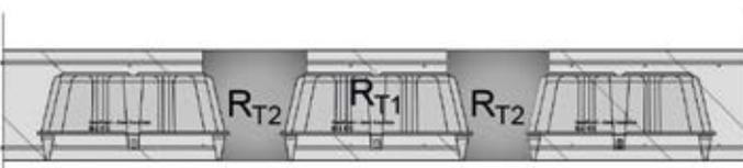
Figure 75 - overall surfaces of thermal resistances in parallel
