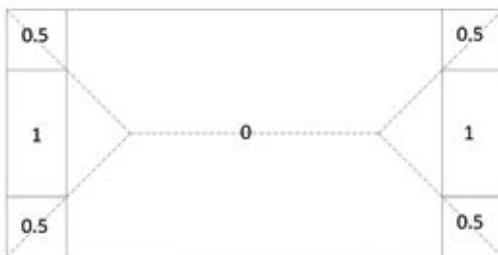
Figura 11 - possible distribution (B) in a rectangular plate leaning on the boundary.
