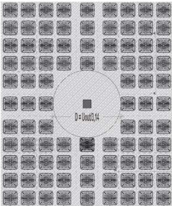
Figure 7 - non-lightened concrete area dimensions - capital
