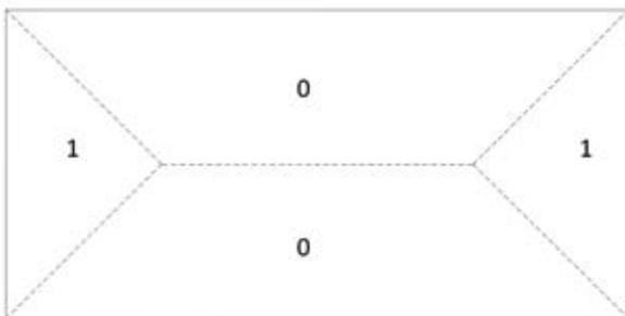
Figura 23 - possible distribution (A) in a rectangular plate leaning on the boundary
