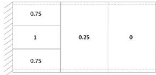
Figura 25 - possible redistribution in a rectangular plate with constraints to mixed
