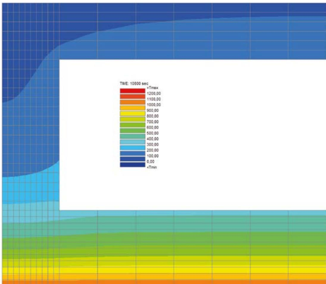
Figure 70 - isothermal configuration for S1 = 80 mm at 180 min
