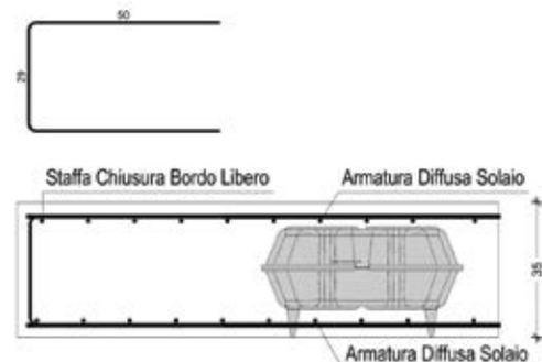
Figure 35 -detail of free edge closing reinforcement
