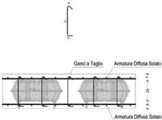
Figura 28 - shear-resistant hooks
