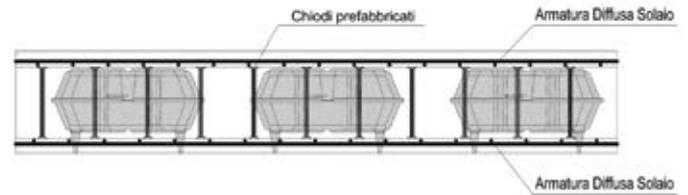
Figura 31 - shear-resistant prefabricated pins
