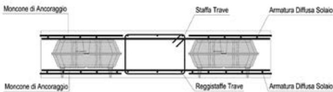
Figure 37 - construction detail of lightening with thick beam
