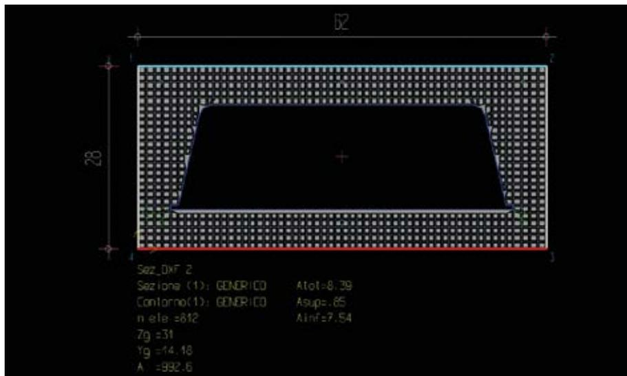
Figure 67 - model F.E.M. of the section
