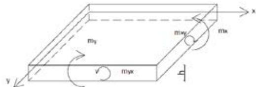
Figure 78 - shear agents on infinitesimal element
