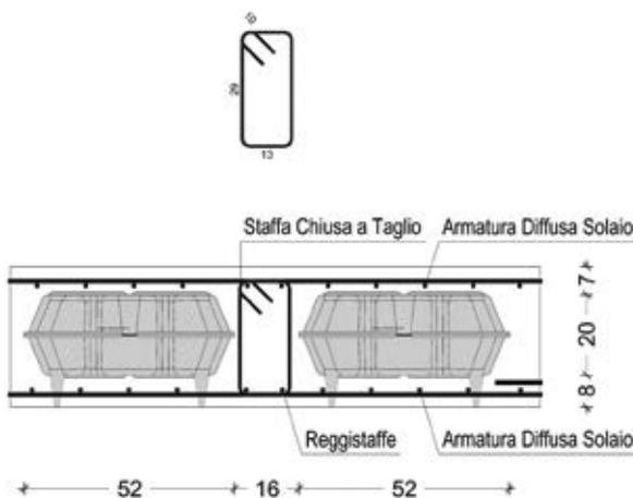
Figura 30 - shear-resistant hooks
