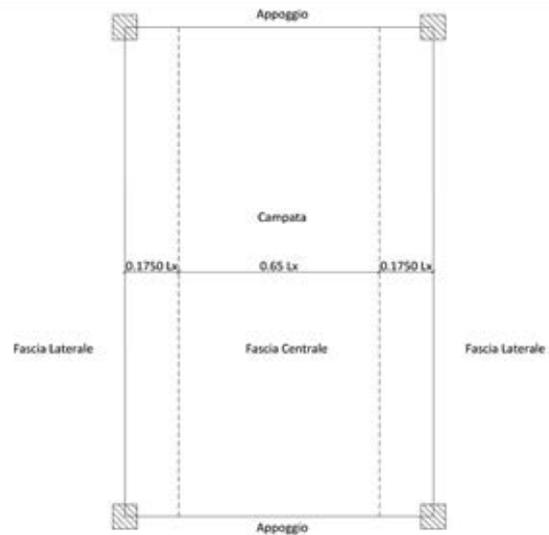
Figura 14 - diagram for the calculation of design moments in the y direction - width of the central and lateral strips.
