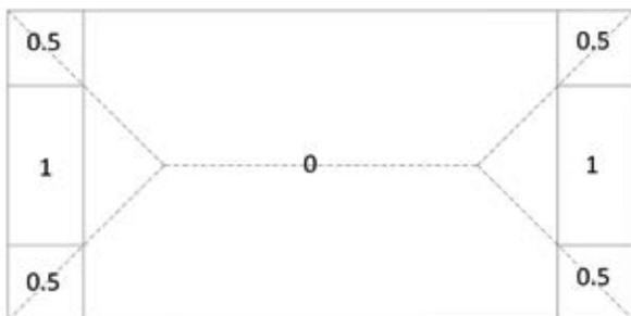
Figura 24 - possible distribution (B) in a rectangular plate leaning on the boundary
