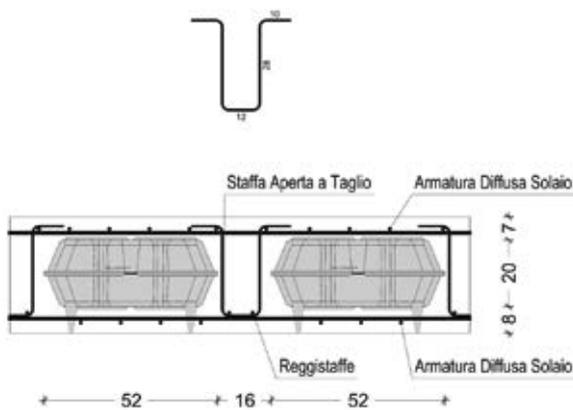
Figura 29 - shear-resistant open ties
