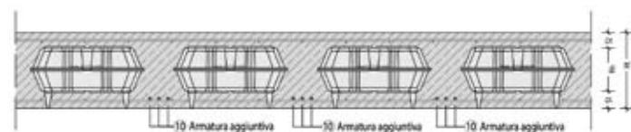
Figure 43 - example of additional reinforcement with loose bars and "double" lightning
