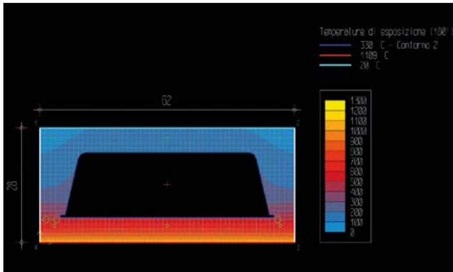
Figure 68 - calculation of thermal conduction over time for application of standardized temperature  $T (^{\circ}C, t)$  curve
