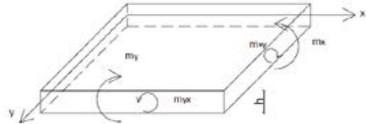
Figure 77 - moments acting on infinitesimal elements
