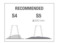
2. Concrete requirements: Use of concrete minimum strength class C20/25. The fluidity class and size of the aggregates must facilitate the filling of the slab below the formwork, depending on its thickness, diameter and spacing of the bars: consult the concrete supplier for the choice of the appropriate mix design. For the first layer casting, we recommend a slump class of S5 and in any case not less than S4. Vibrate the pour appropriately to avoid segregation and gravel nests.
