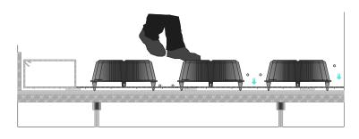
Construction site staff can walk directly on the void formers. Additional reinforcement, and shear stirrups may be laid.
