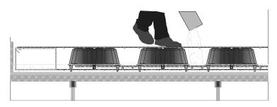
In order to avoid floating of the void formers, the casting process should be divided into two step: in the firs step the cast reaches 2 cm above the footing maximum. Properly vibrating, concrete flow under the void former may be checked through the central hole.
